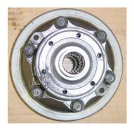
3. Remove the six bolts, then place the differential assembly with the housing side down, and remove the ring gear.
