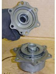
4. Once bolts are removed you will find 1spring washer, 1 concave spring washer, 1 side gear. Set these items aside.
